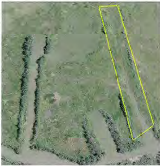
Fig. 3. A canal backfilled in 1981 is outlined in yellow. Compare the area of vegetation in the canal and the spoil bank vegetation on the former spoil bank with the area of vegetation for the canal to the left that was not backfilled.
